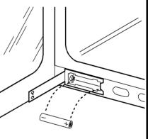
When you fit the new battery, make sure the positive end (marked with a + sign) is next to the (+) sign on the battery holder. Close the lid of the battery holdler.
